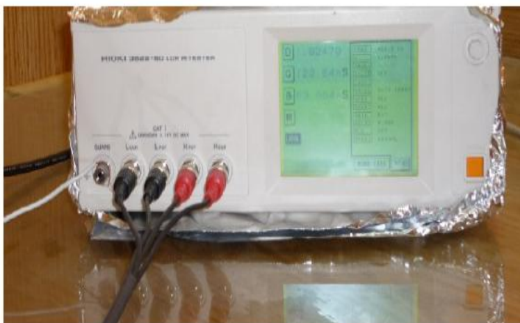
Fig 1: Life photo for experimental HIOKI 3522-50 LCR Hi-tester device equipment's
